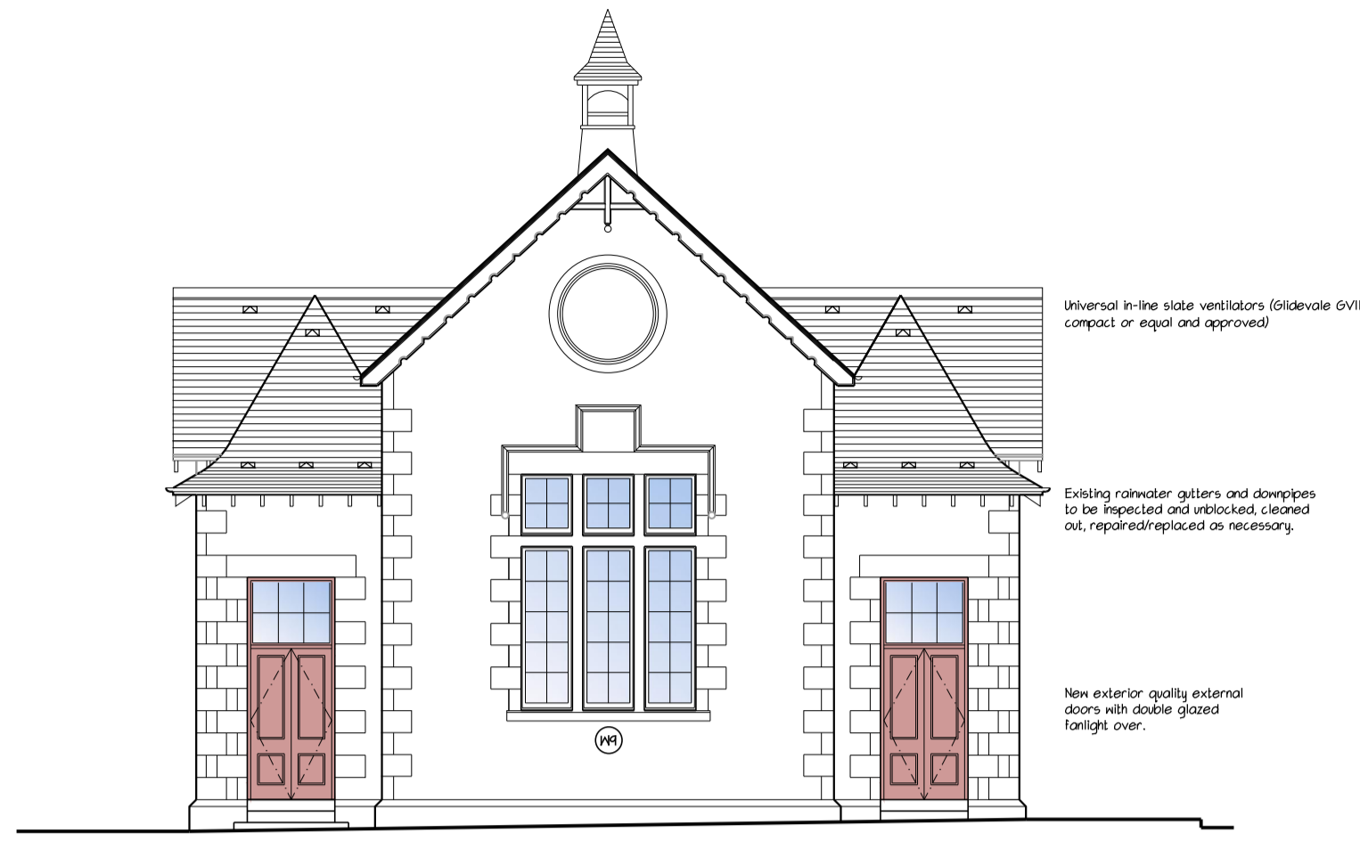
NORTH WEST ELEVATION
